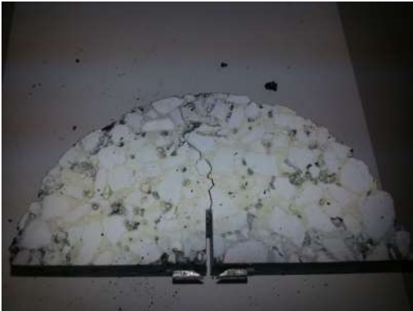
SCB Fracture Test at Low Temperature (-12C) Rate (6.25mm/min)
