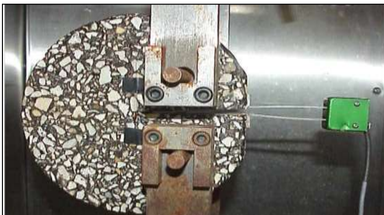
Disc Compact Tension (DCT) @ Loading Rate = 1.0 mm/min
