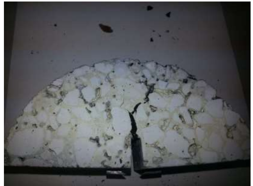
SCB Fracture Test at High Temperature (25C) Rate (6.25mm/min)
