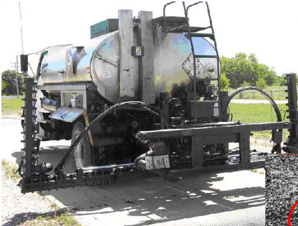
Centennial variable-bar liquid distributor
