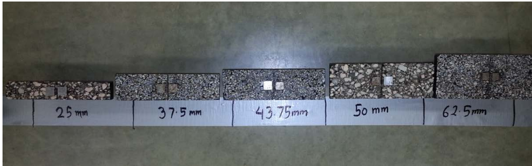
Figure I.1 Variation in thicknesses from 25 on the left to 62.5 mm on the right.
