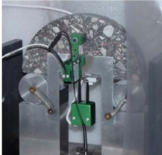
Figure 2.3 Semi-circular bending beam test fixture and typical outcome from this test to calculate fracture energy (Marasteanu et al. 2012).
