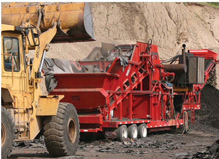
Figure 5-1. Shingle grinder (left) and rotating Trommel screen (right) used for RAS processing.
