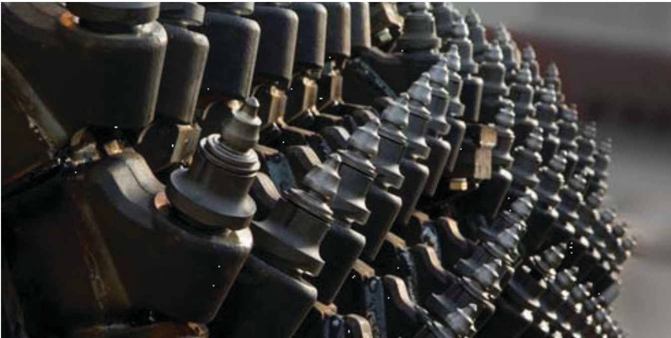
Figure 1-4. Micro-milling drums have three times the number of teeth as a normal milling drum.
