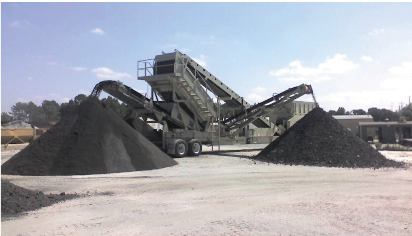
Figure 2-7. Portable RAP fractionation unit. This unit screens RAP into three sizes: + \frac{3}{4} " on right, - \frac{3}{16} " on left, and \frac{3}{4} " x \frac{3}{16} " in back.
