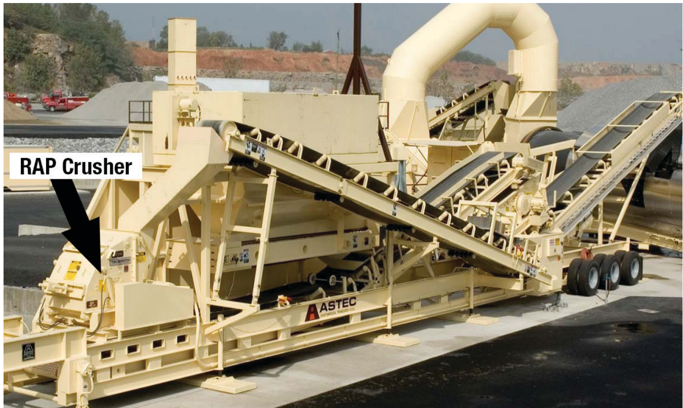
Figure 2-4. RAP processing unit with a screen before the crusher.
