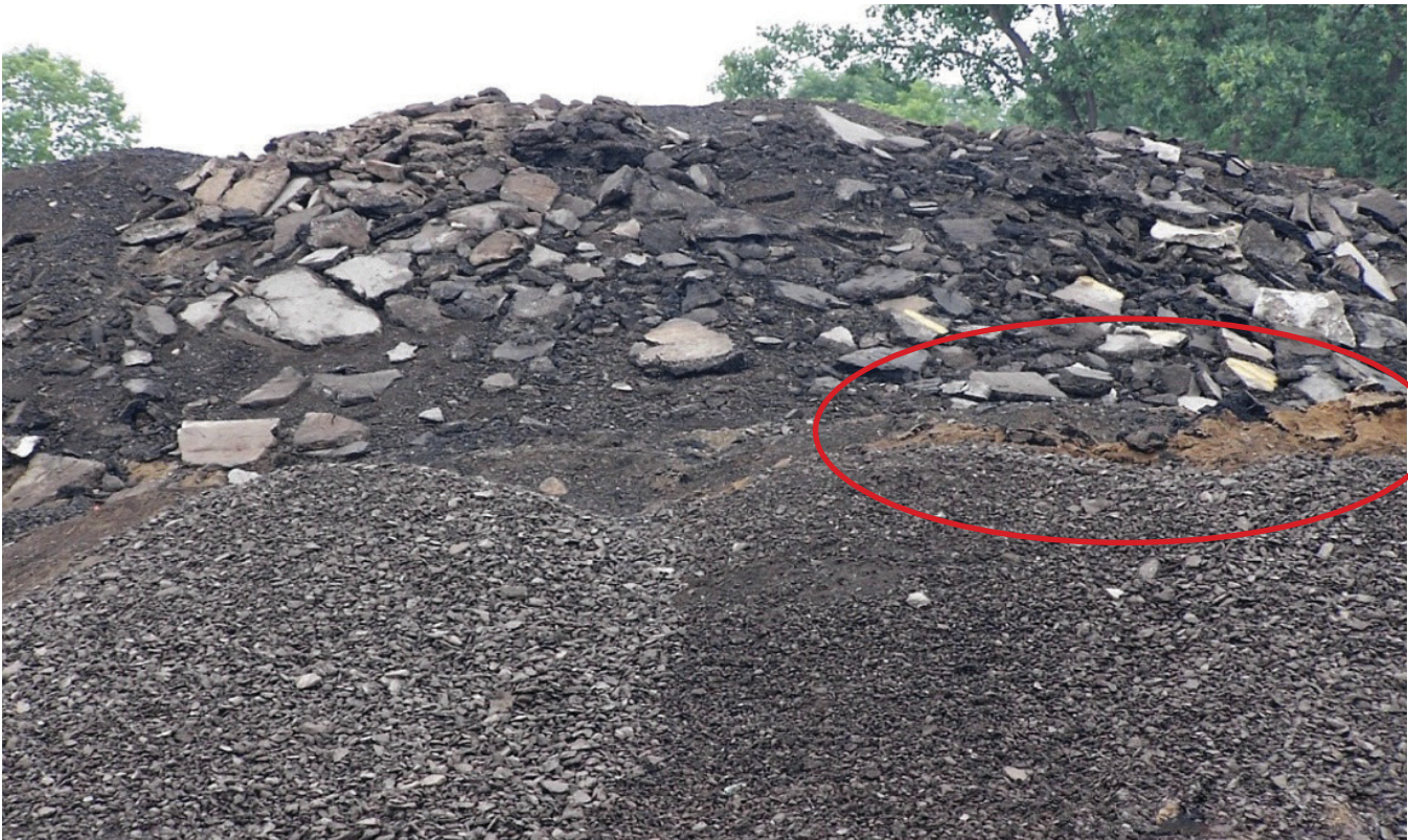
Figure 1-6. Multiple-source RAP pile with dirt contamination (circled in red).
