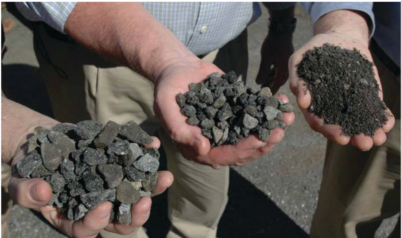
Figure 2-6. Samples of fractionated RAP.
