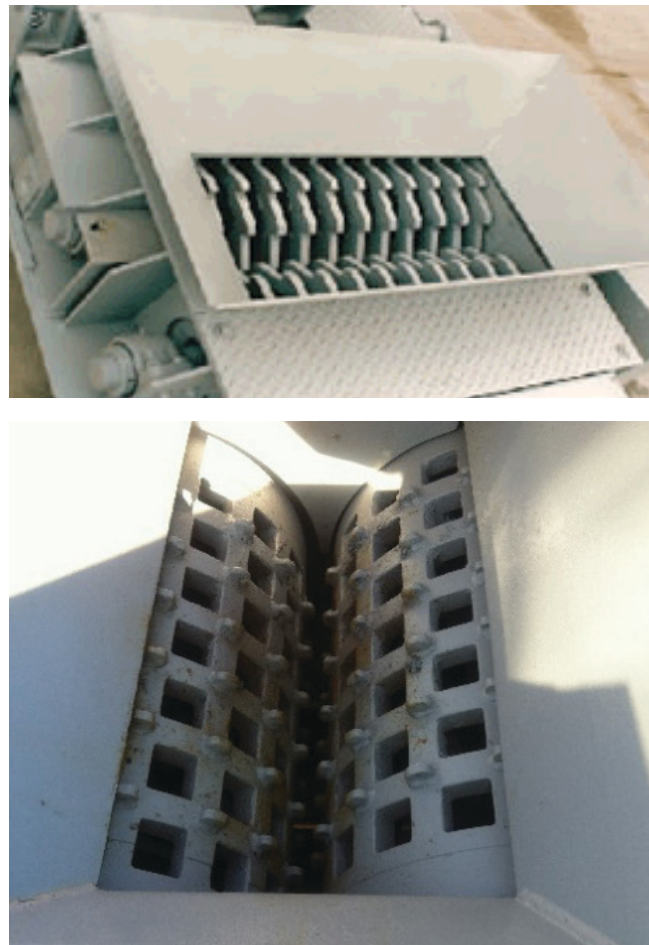
Figure 2-10. Roller crushers designed to break up agglomerations of RAP.
