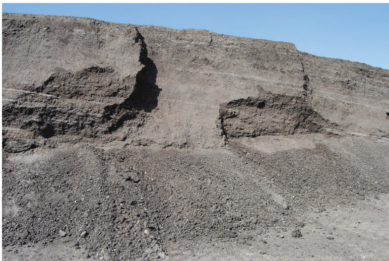
Figure 2-2. Working face of a stockpile of milled RAP. Layers of the materials are evident.
