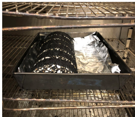
Figure 3 – Example of test specimens ready to undergo aging conditioning.
