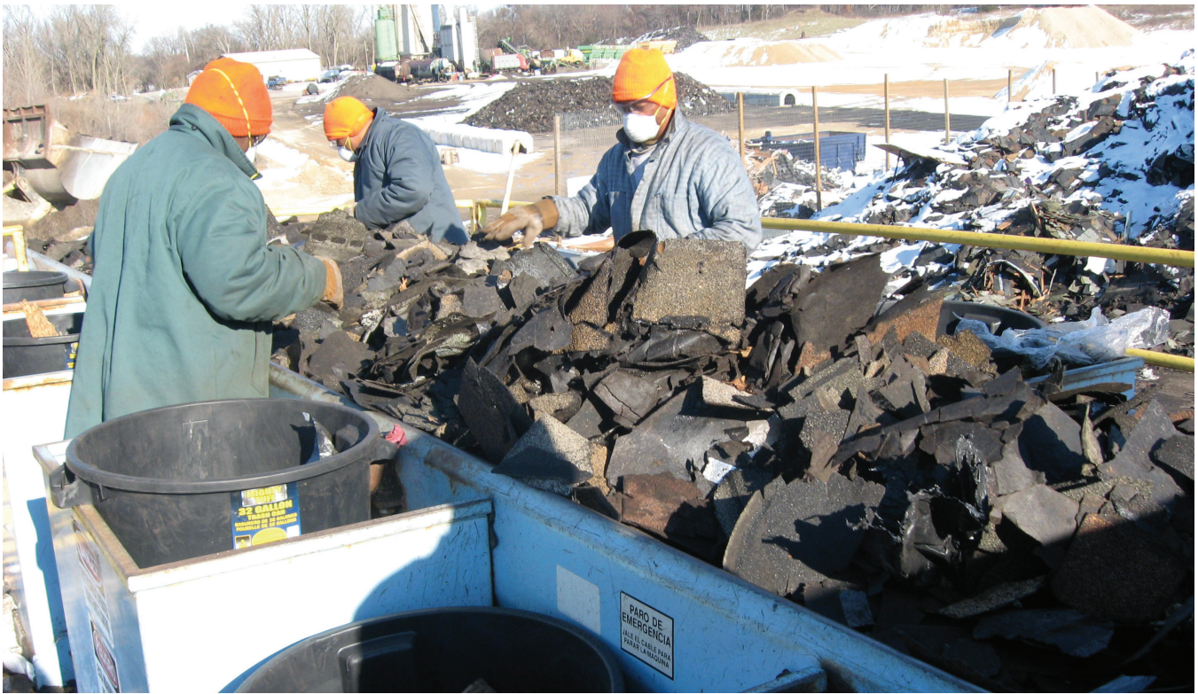
Figure 5. Shingle Sorting Operation (courtesy B.R. Amon & Sons Inc.)
