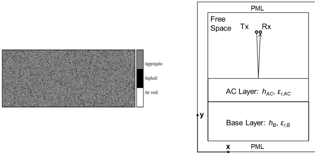
Figure 2 the three-phase asphalt mixture numerical model.
