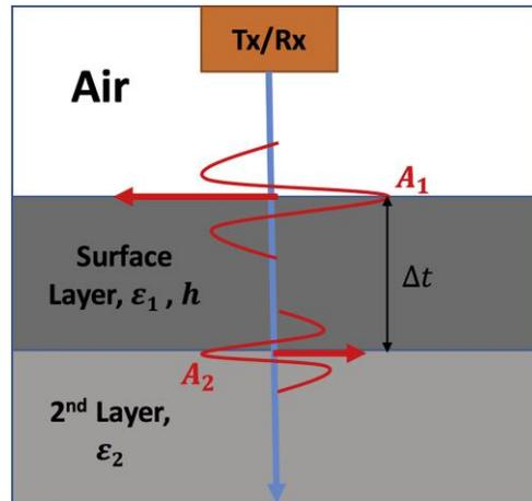
Figure 1 GPR signal reflected from a two-layered AC pavement
