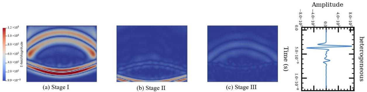
Figure 3 simulated signal in GPR measurement.
