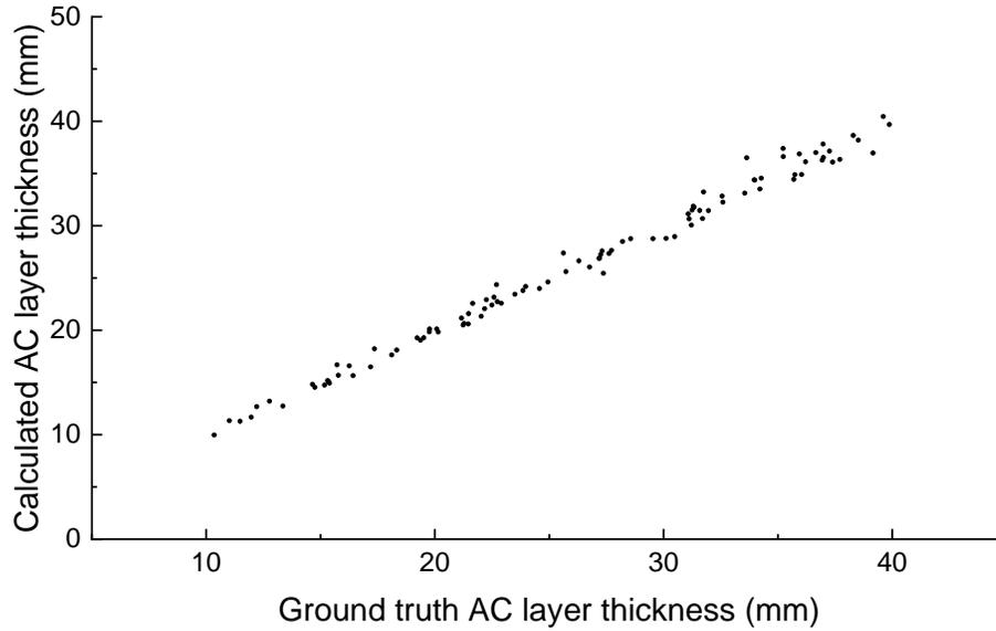
Figure 5 calculated thickness in the numerical simulation of thin overlay.
